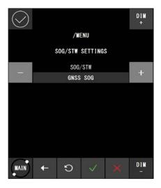
GNSS SOG: Speed over the group by the satellite log (initial value)
