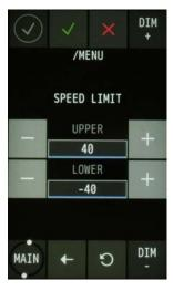
When the [-]/[+] button on the screen is touched, each of [UPPER] (upper limit) and [LOWER] (lower limit) decreases/increases. OFF cannot be input with the [-]/[+] button. The [UPPER] cannot be lower than the [LOWER], and the [LOWER] cannot be more than the [UPPER].
