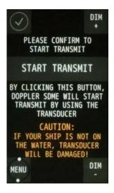
When the [START TRANSMIT] button is touched, the normal screen is displayed. Transmission starts.
