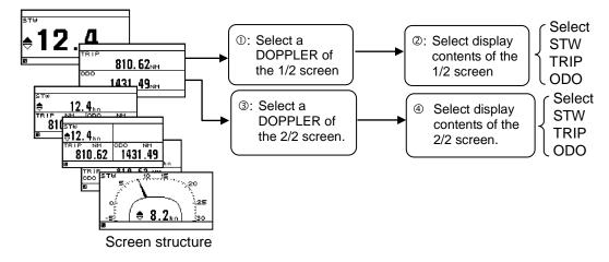
1 Select a screen structure by referencing "STEP1" and "STEP2".
