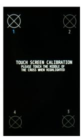
3 Touch the center of the target marks at the four corners of the screen.
