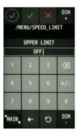
When a numeric digit that has been input is deleted, OFF is input.
